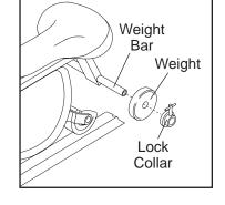
on each side of the weight bar. The total combined weight of the user and added weights should not exceed 300 pounds.
